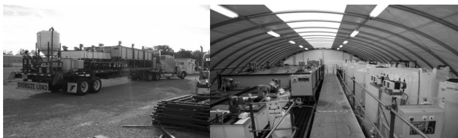
Figure 5: Portable 40-117 L/min AMD VEP™ F-LLX™ field demonstration unit
